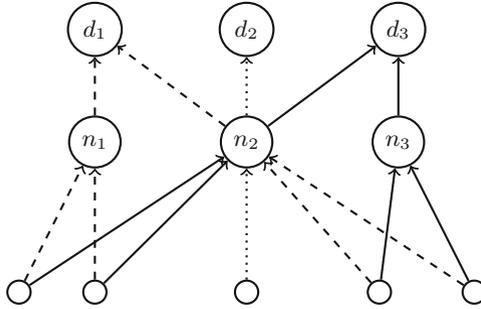
**Fig. 3.** Sample network with 3 domains, 3 nodes and 5 sources. The dashed lines are channels to domain  $d_1$  the dotted line is the channel to domain  $d_2$  and the solid lines are channels to  $d_3$ .
